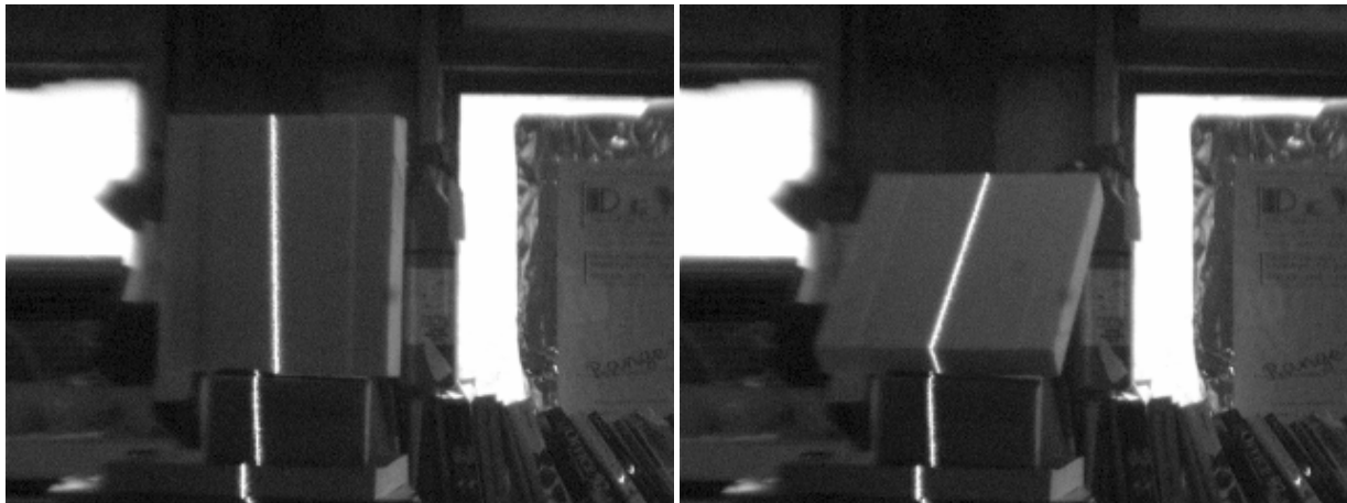
Figure 6 Zero-order images of vertical and 45 degree test blocks created by using a mirror in place of the grating. The structured illumination spill below the test blocks illuminates a supporting pedestal and does not appear in the diffraction images of the same targets in Figure 7.
