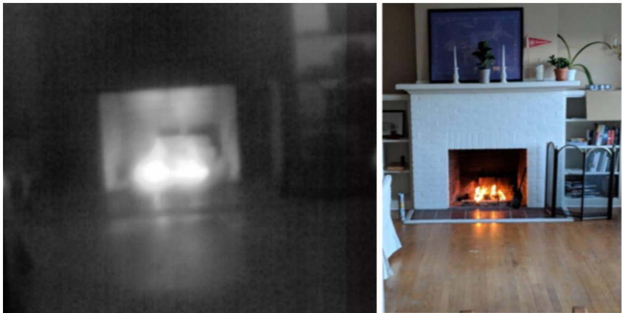
Figure 4.3-1: Fire shown with thermal imaging Seeker Thermal 206x156 (Left) Google Pixel 2 3024x4032(Right)
