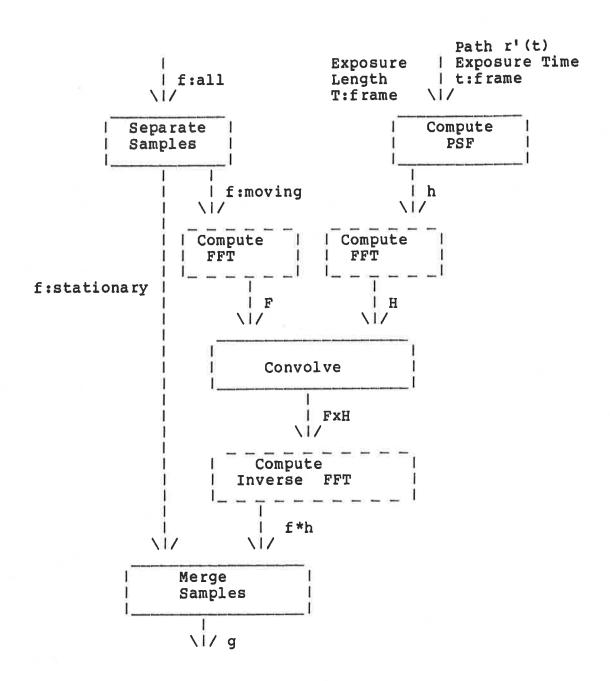
Figure 1 Block diagram of the motion-blur processor
