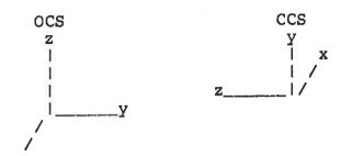
Positive rotation is clockwise motion about the named CCS axis as if you were looking toward the origin while sitting on the axis. Initially the camera positioned at point (0,200,0) in OCS will point towards (0,0,0) in the OCS iff dx,dy, and dz are 0. The camera therefore looks out its own z axis. This is translation and rotation independent, the camera always looks down the CCS Z axis. From the initial camera position the grammer for camera is as follows:
