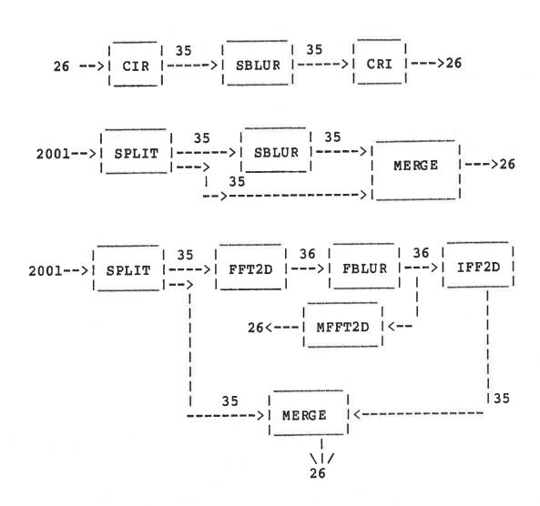
Figure 3 Typical paths to generating motion blur
