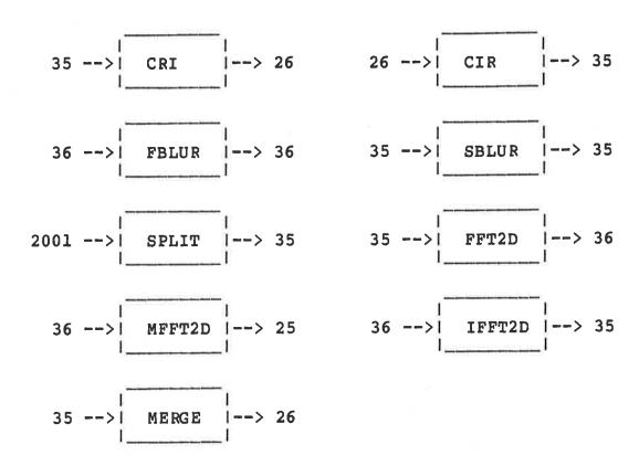
Figure 2 Image type before and after applying an operator
